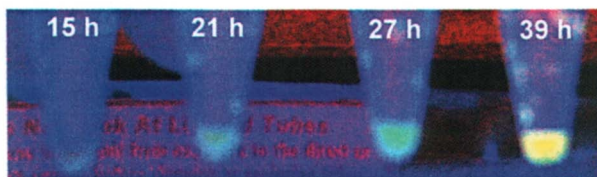
Figure 20.2. Luminescence increase and color change of the hybrid T_7 -A/MAA CdTe QDs depending on the duration of reflux.
